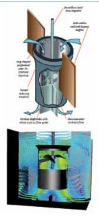
Figure 2: Computational fluid dynamics (CFD) is helping system designers to more effectively build better wastewater treatment systems.
