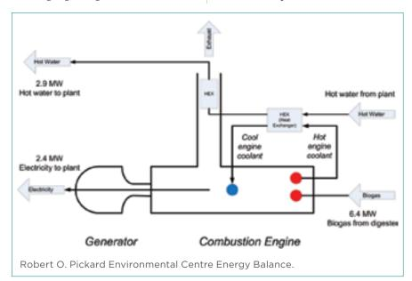
digester gas-fuelled CHP plant continuously for more than 12 years. Given the nature of the fuel, known for its corrosive contaminants, the Caterpillar model G3516 low emission engine-generator sets have performed remarkably well, each with more than 100,000 running hours, and demonstrating the benefits of being purposefully designed to withstand corrosive attack, fluctuating fuel energy quality, and unattended operation.
