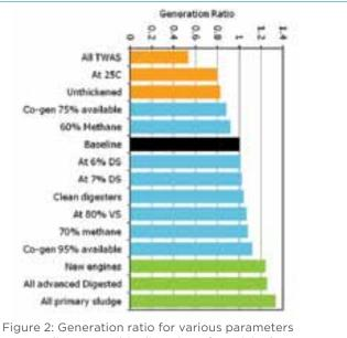
Figure 2: Generation ratio for various parameters surrounding anaerobic digestion of municipal sewage sludge. Green bars are parameters that increase energy generation above 20% and orange bars reduce generation by approximately 20%. The black bar is baseline.
