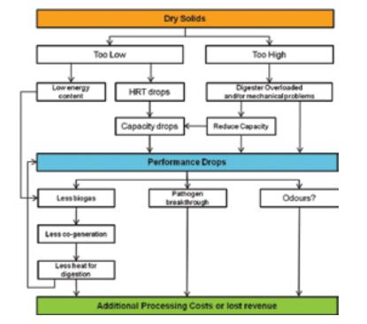
Figure 3: Impact of dry solids content on anaerobic digester performance.
